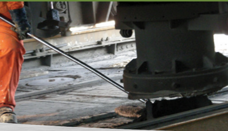
Figure 8. Lidman replaces the lid after the coal has been charged into the battery
